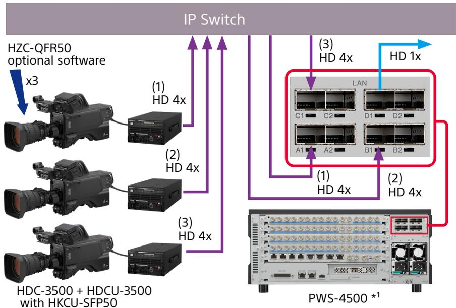
\*1 The optional PWSK-4509 ST 2110 Interface Board and PWSL-HF45 HFR (High-frame-rate) Software are required.
