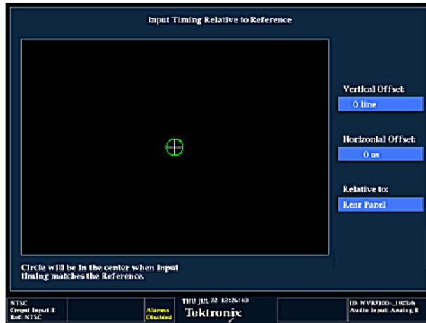
If you time input rates that are not integer multiples of the reference rates, the instrument cannot measure the timing deterministically, so it displays the relationships as several circles. Each circle represents a possible timing offset measurement relative to the reference cross-hair. Display emphasis is given to the circle that times closest to zero offset and the numerical readouts track this pair.
