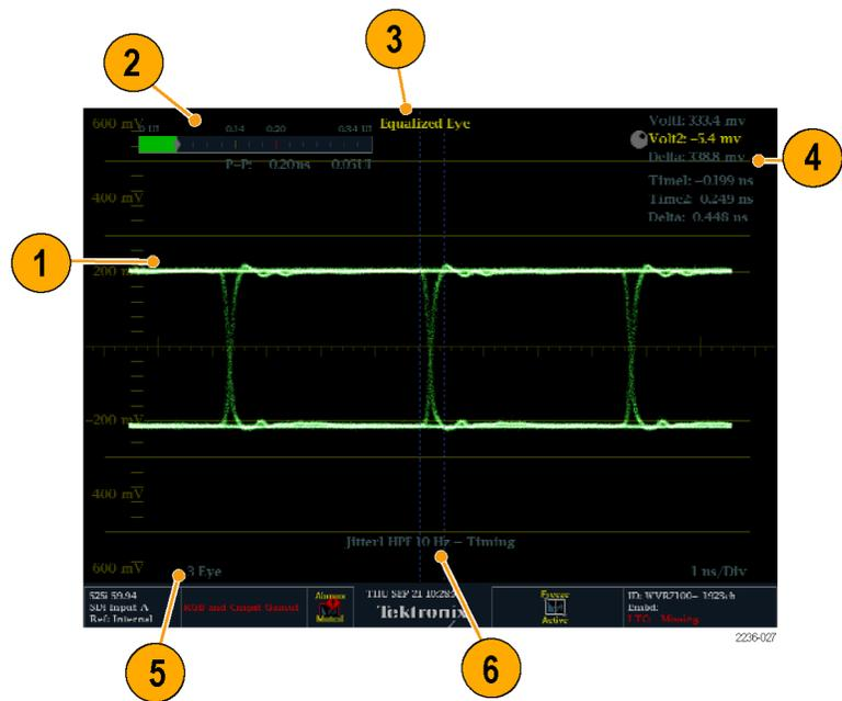
At the end of a long cable, the eye diagram may appear so noisy that there is little or no discernible opening. In this situation, limited use of the eye diagram is still possible by selecting Equalized Eye mode. The equalizer compensates for the effects of cable length by applying an inverse response function and then reslicing the signal to a logic level. This causes amplitude information to be lost, but preserves the effects of jitter in the signal.
