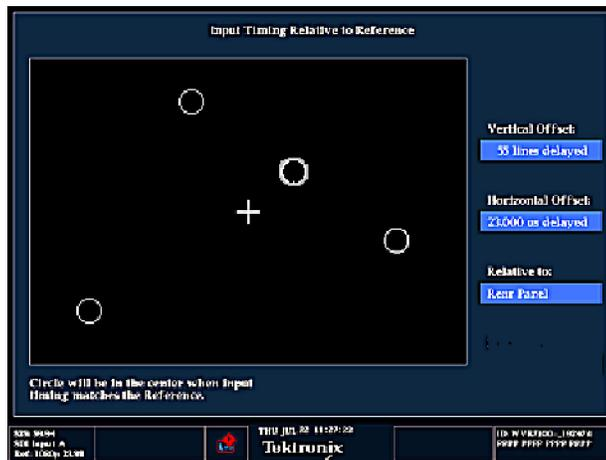
For a case where multiple relationships would display, consider an input of 1080p/23.98 Hz with a reference of NTSC/59.94 Hz:
