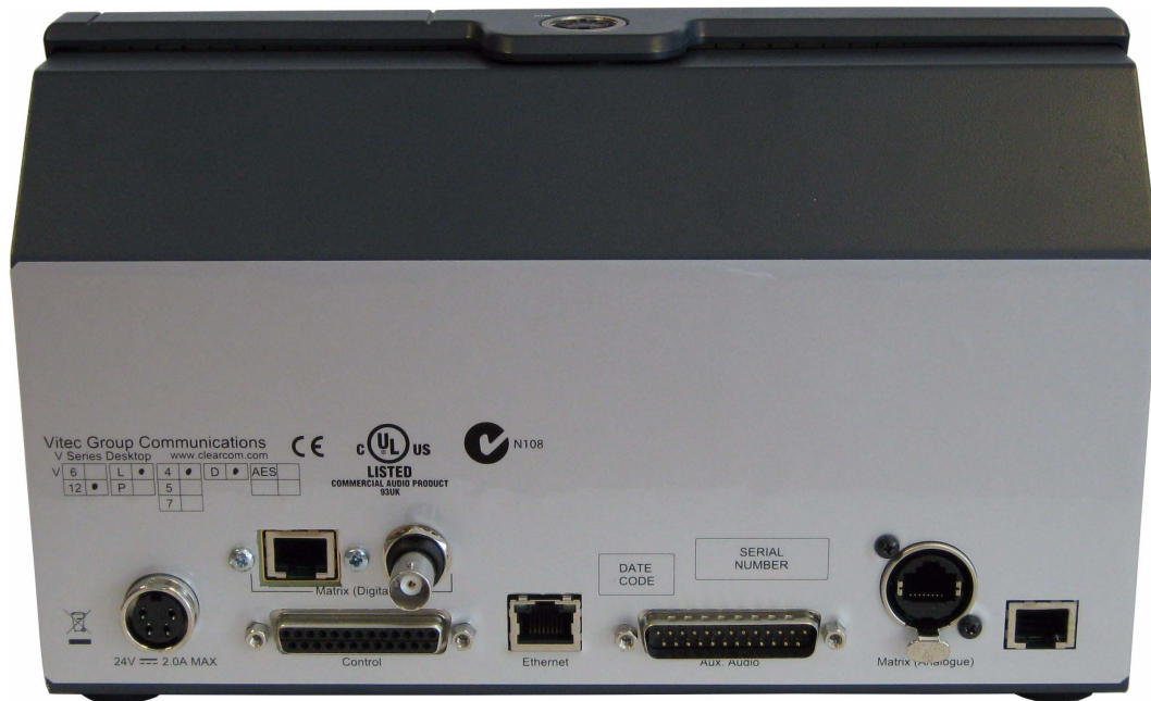
Figure 25: Completed Desktop Panel Upgrade with AES-3
