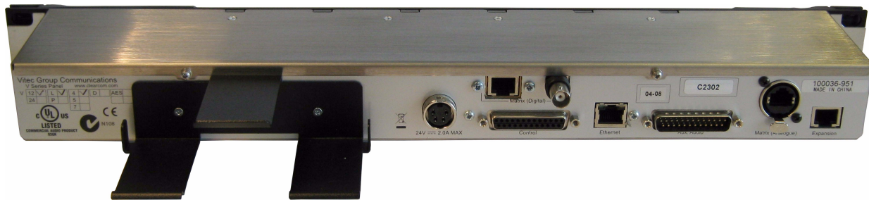
Figure 13: Completed Rack Mount Panel Upgrade with AES-3
