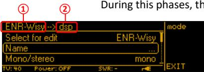
During this phases, the name of the MODE to edit appears on the left top of the display ①. If the MODE to edit is the current mode loaded on DSP (on the Main>Mode menu), “dsp” abbreviation is shown ②.
