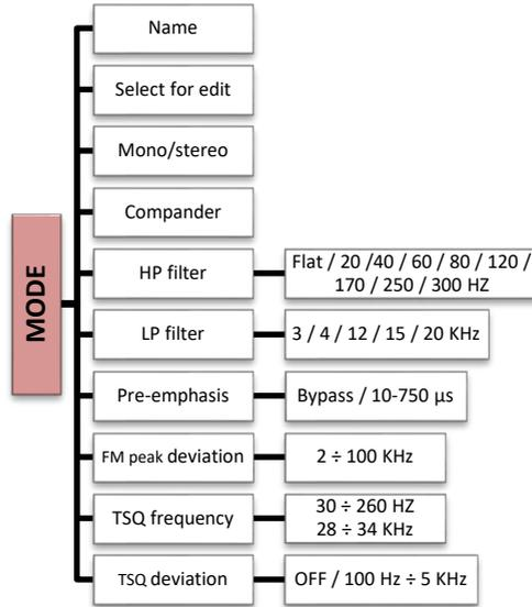
To access the configuration menu of the transmitter is necessary to press the rotary knob (at the right of the display ①).
