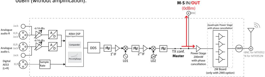
When the MTK952N is in Slave configuration, everything that is before the power stage is excluded and the device take as input the signal that enter in the M-S I/O BNC connector, amplifies the signal (at the power set on the MTK952N-Slave) and transmits it.
