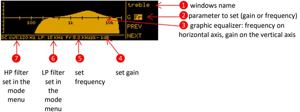
For each window it is showed the graphic equalizer which help to see the set parameters. Push the rotatory knob to change the parameter between gain and frequency (the respective letter **G** or **Fr** is highlighted during the setting phase) and
