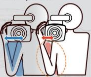
By reducing the width of the drive unit. the palm of the camera operator's hand is positioned closer to the optical axis, thus reducing the degree of arm bend which in turn lessens physical stress during prolonged shooting.
