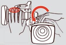
The spacing between the focus ring and drive unit has been changed to avoid accidental interference with the drive unit while manipulating the focus
