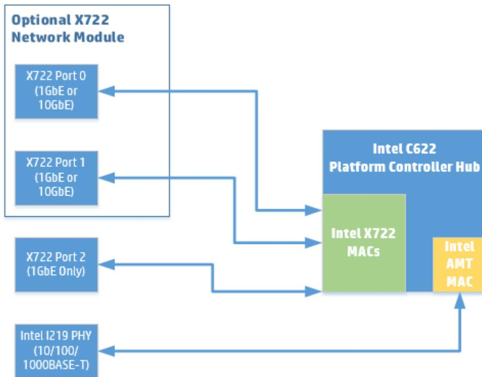
**Note:** When an optional X722 network module is not installed in the system, a “dummy” port is enumerated as Function 0 of the Intel X722 MACs, which allows for the X722 Port 2 on the Motherboard to enumerate.
